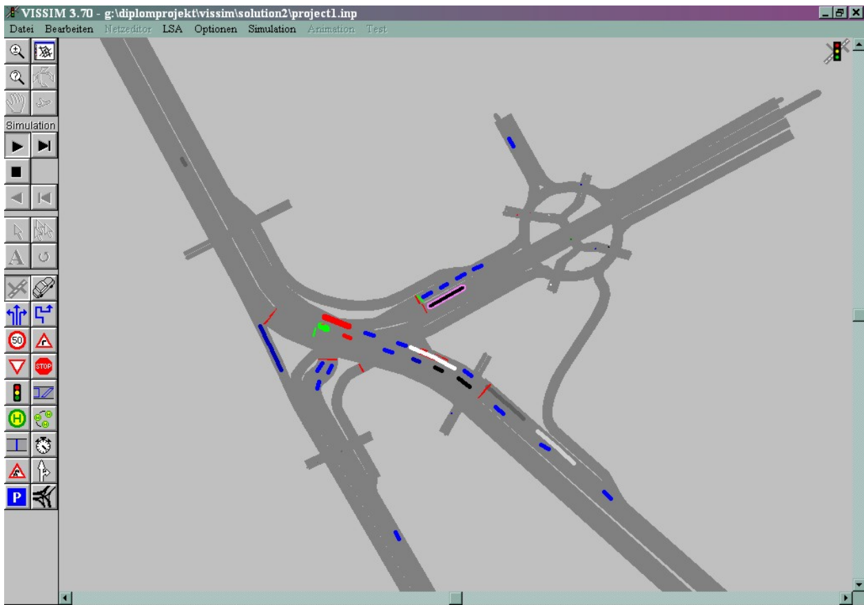
Fig 1. The run of simulation of the signalised intersection Lenina St.-Sedova St. (Irkutsk)
